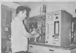
Lab Assistant Mario Croes datamines the ppm of sulfur in liquid pentane feed sample using Wickbold combustion procedure. Lab Assistant Mario Croes ta datamina contenido di azufre den pantana for di Hydrogen Plants usando Wickbold machine.
